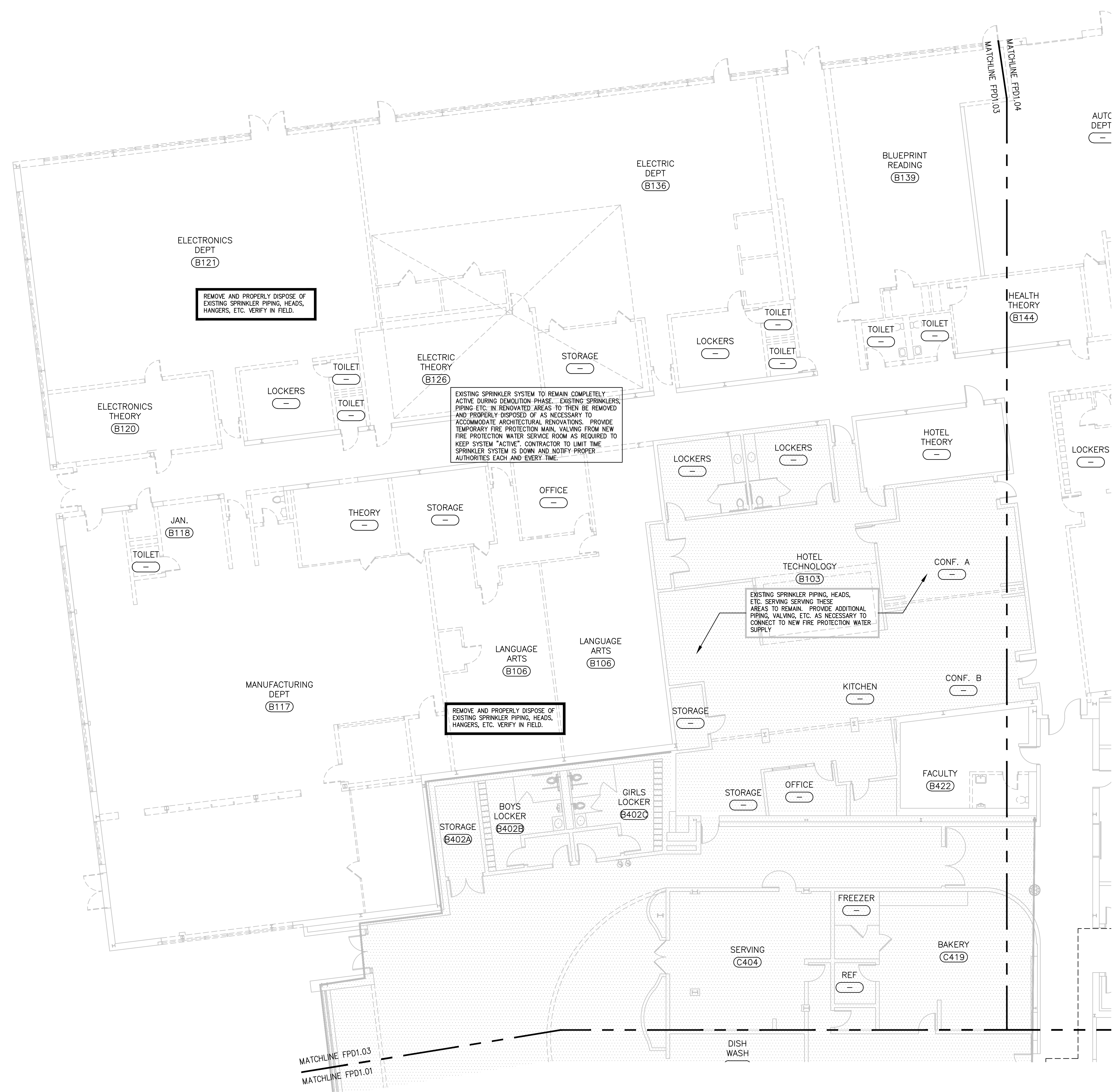
1 FIRST FLOOR DEMOLITION PLAN - AREA "B" & "C" FPD1.03 1/8"=1'-0"
