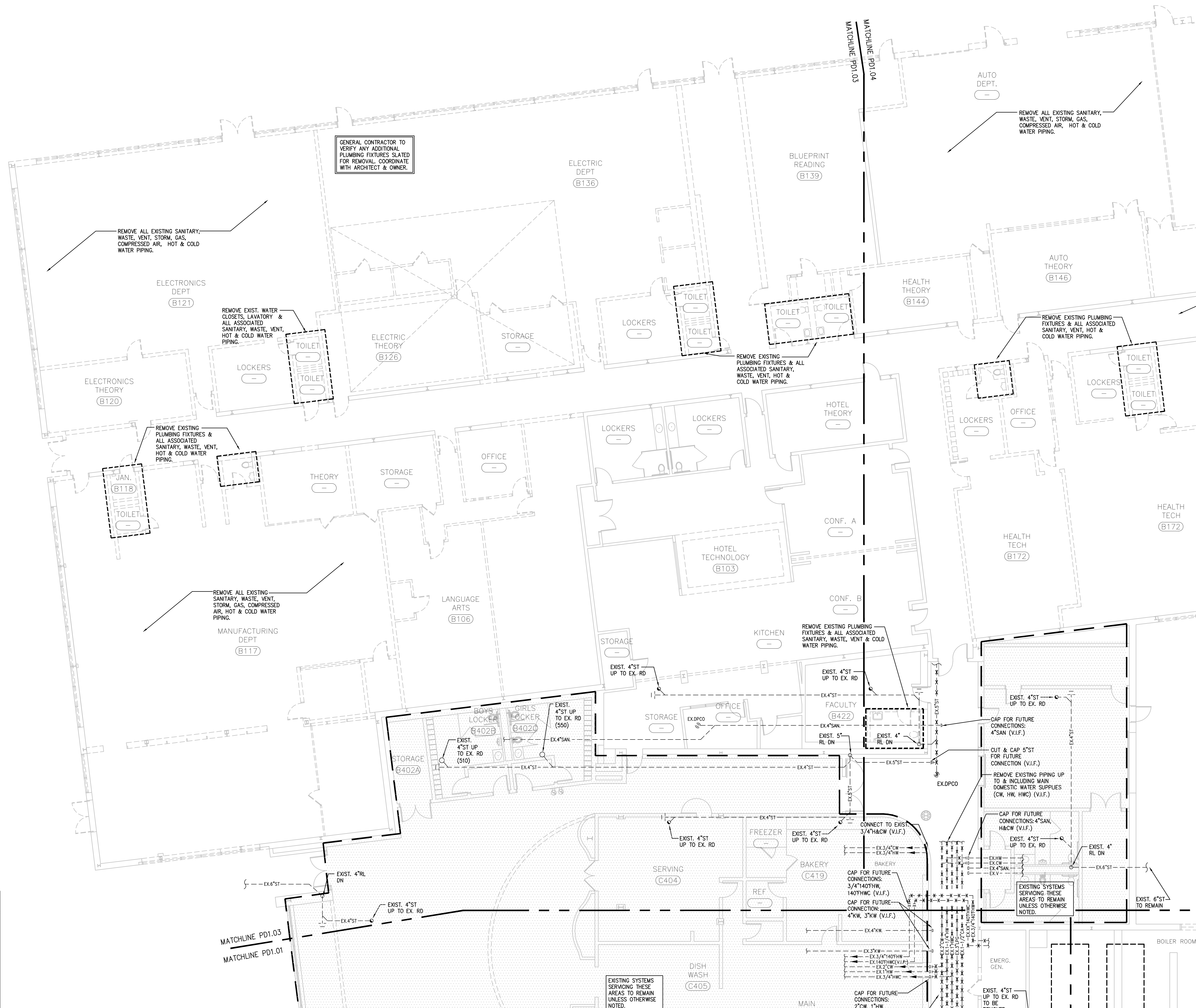
1 FIRST FLOOR DEMOLITION PLAN - AREA "B" & "C" PD1.03 SCALE: 1/8"=1'-0"
